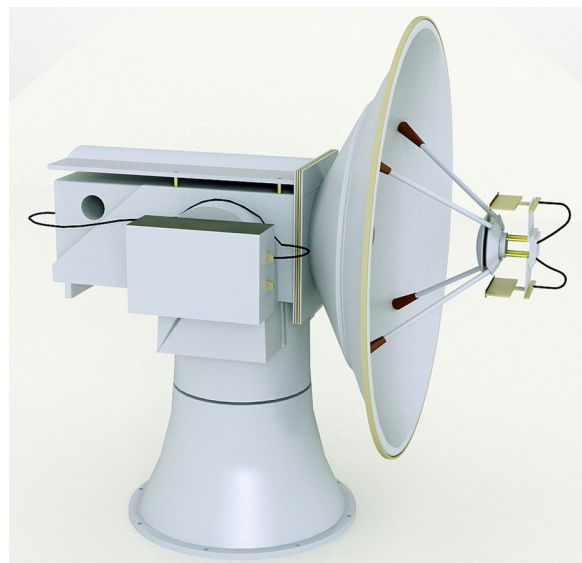
Radar antenna 35 GHz
